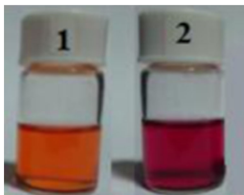
Fig. 3 The color change of the sensor upon complexation with \text{Hg}^{2+} ions (1 ATBD; 2 ATBD + \text{Hg}^{2+} )
